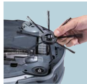
Side Brushes are designed to help capture debris alongside walls, corners and obstacles
